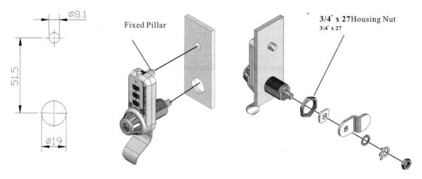
VI . When the finger pull is not installed, please add one flat washer to assist the lock to fix
