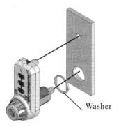
VII · Please note, before installing the cam, please turn the wheels to the correct combination code, and then tighten the cam by hex nut. Please comply with these steps when installing to ensure the internal components functions normally."
