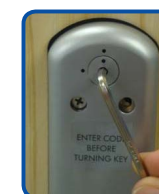
Turn the code change cam on the inside handle from the 9 o'clock positioned black dot to the 12 o'clock positioned black dot.
